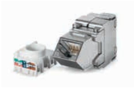
RJ45 module KS-TA 1/8 Cat. 6/E A , shielded, 45° angled
