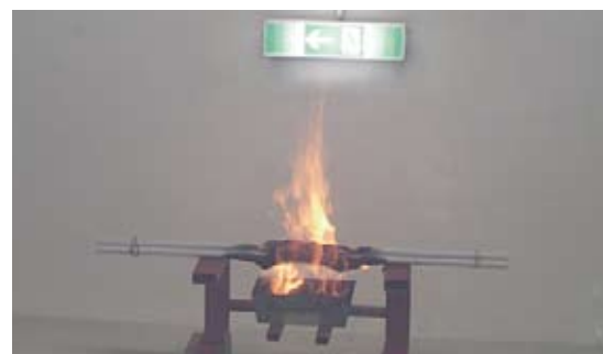
Fire test with FPKu-EM-F-LS0H
