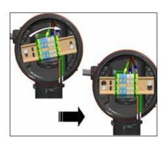
**13.** Install terminal block and complete system wiring. Terminal set screws shall be tightened to a torque value of 1.4 Nm (12.4 lb-in). See below for wiring details.
