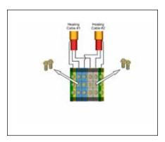
End Termination (1 to 2 Heating Cables) Remove jumpers for 2 cable terminations.
