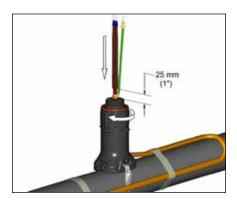
**9.** Push excess cable back through expediter. Tighten cap securely. Tape cable expansion loop to pipe.
