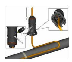
Insert cable into expediter. If mounted on bottom or side of pipe, punch out weep hole
