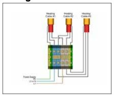
Power Connection (1 to 3 Heating Cables)
