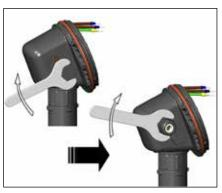
11. Remove M25 dust cap. Install M25 power gland (order separately) and M25 blind plug. For in-line splice, T-splice, or end termination, install additional M25 blind plug (order M25-B-EXE separately) instead of M25 power gland.
