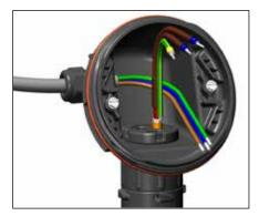
**12.** Install power cable (if necessary).
