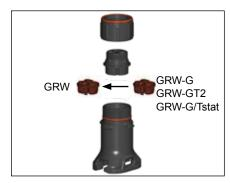
For HPT and FP cable exchange grommet supplied in Terminator kit with: GRW-G provided in PETK-3 GRW-GT2 provided in PETK-3-ECM GRW-G/Tstat provided in PETK-3-ZT
