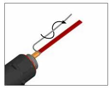
1c. Twist braid into a pigtail. Trim ends of
