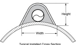
Typical Installed Cross Section (TFK channel and heat transfer compound shown covering tubular heater or tracer)
