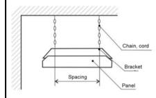
Spacing of grips at the back side of the panel: After insertion, it is advisable to secure it in position with the use of positioning screws to prevent it from sliding out.
