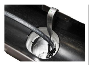
The cable releases a significant amount of power when exposed to snow and icy water (36 W/m @ 0°C). When the ice has melted and the cable is dry, the heating effect is reduced by half, which provides significant energy savings.
