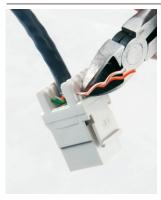
Use an appropriate wire cutter to cut off the excess lenght of the wires
