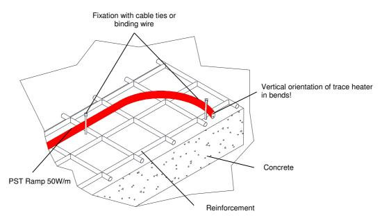
The maximum allowed heating circuit length must not be exceeded! Instead, add another heating circuit if required! Install the end termination kit as soon as possible; Under all circumstances avoid ingress of water or moisture in the trace heater. Fix end termination to reinforcement via cable ties. Trim cable ties along the entire trace heater. Repeat the above listed steps for all heating circuits.
