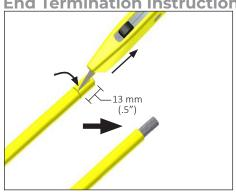
Cut and remove heating cable overjacket.
