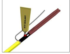
Apply RTV sealant to cable to cover distance of at least 4 mm (1/8") and slide boot onto the end of the cable.
