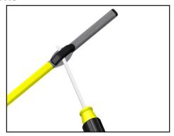
Separate braid strands at edge of overjacket and pull cable through opening in braid.
